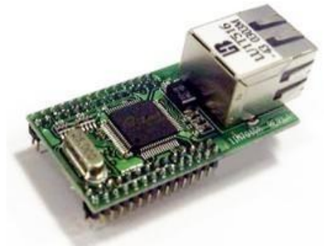
Fig: An example of a COTS product for TCP/IP plug-in from WIZnet (WIZnet NM7010A Plug in Module)
