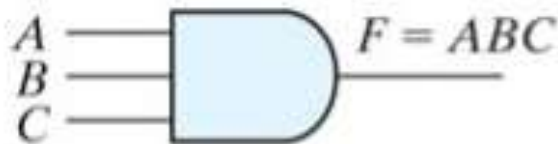
Three-input AND gate
