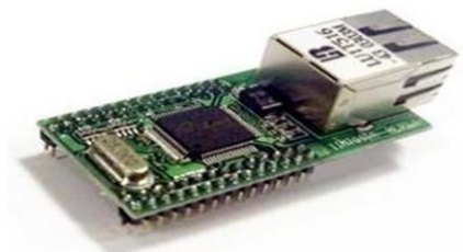
Fig: An example of a COTS product for TCP/IP plug-in from WIZnet (WIZnet NM7010A Plug in Module)
