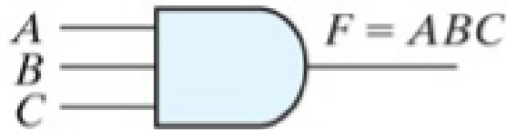
Three-input AND gate
