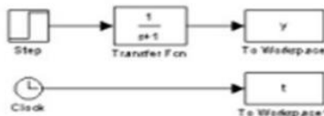
Fig. 10. Block diagram for Workspace displaying
