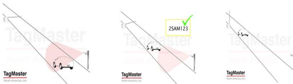
In an LPR application, the vehicle's license plate serves as its identification credential, eliminating the need to administer any additional credentials or mount any tags to the vehicle. An LPR camera's job is to capture an image of the vehicle's license plate, and use the plate image to accurately process and identify the license plate characters. The camera can then forward the plate ID information to an access or revenue system.
