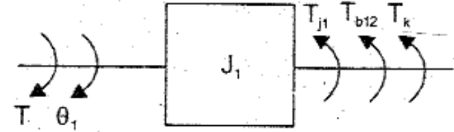
Fig 2 : Free body diagram of mass with moment of inertia J_1 .
