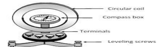
Tangent Galvanometer
