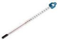
Measuring temperature by measuring length
