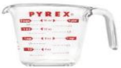
Measuring fluid volume by measuring height
