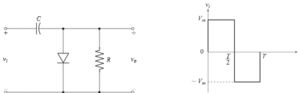
Fig.1.13: Negative clamper circuit.
