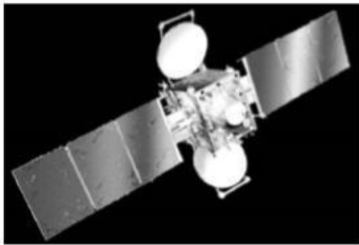
Fig.2.3 Flat solar panels used on three-axis stabilized satellites
