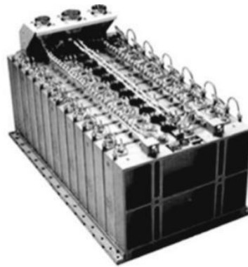
Fig.2.6 Nickel-cadmium battery pack used on SPOT-4 satellite
