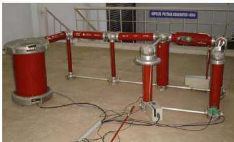
Fig. 2. Basic circuit of single stage impulse generator
