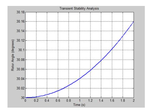
Initial Acceleration Power: 0.00 p.u. Acceleration Power After Fault: 0.40 p.u.
