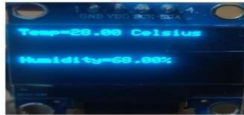
Figure 2.4: Displaying Temperature and Humidity values on OLED using Arduino
