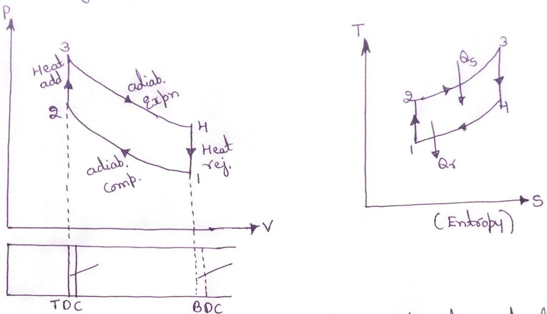
Let the cylinder contain  $m \text{ kg}$  of air at its initial condition represented by point 1 on p-v and t-s diagrams.
