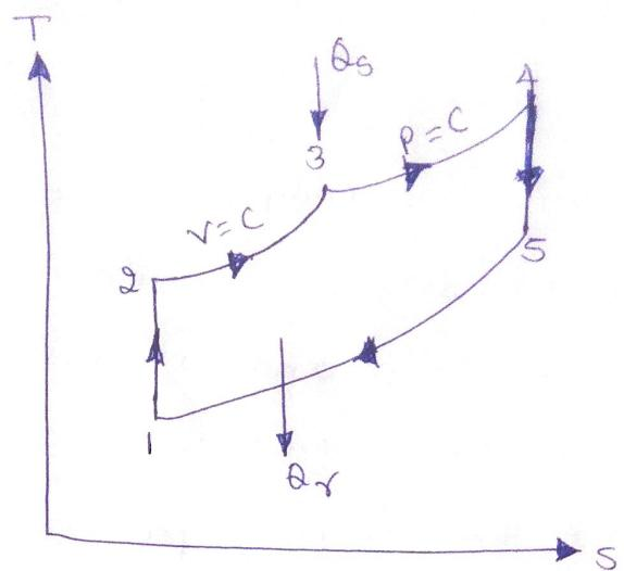
Let the cylinder contain  $m \text{ kg}$  of air at its initial condition represented by point 1 on p-v and t-s diagrams. The dual combustion cycle consists of the following processes.
