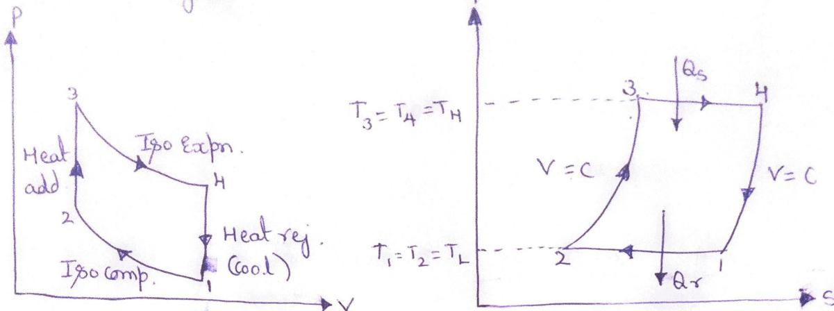
Let us consider  $m$  kg of air at its initial conditions represented by point 1 on P-V and T-S diagrams. The various processes involved in Stirling cycle are discussed below.
