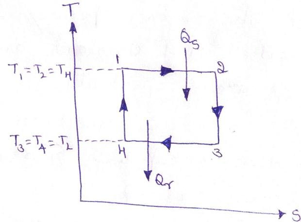
Let the cylinder contain 'm' kg of air at its initial condition represented by point 1 on p-v and t-s diagrams. The various processes involved in Carnot cycle are discussed below:
