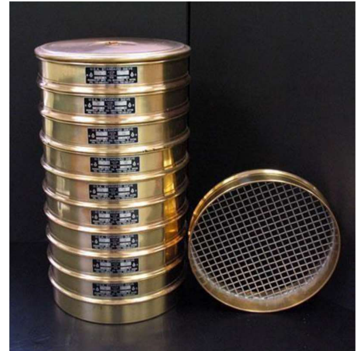
Stacked sieves used for a gradation and size test
