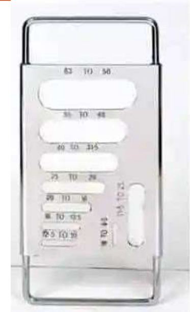
Flakiness Index- Thickness Gauge
