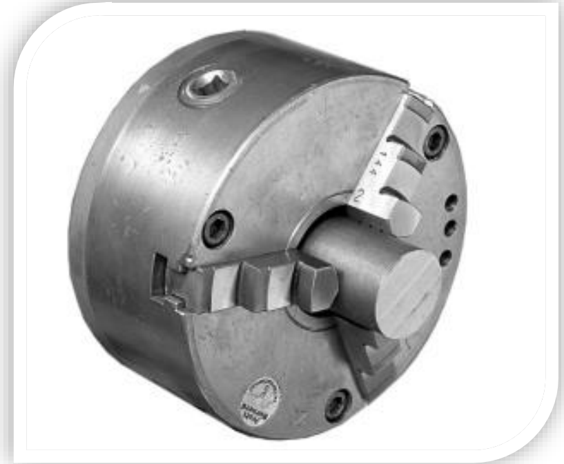
Three-jaw universal chuck.
